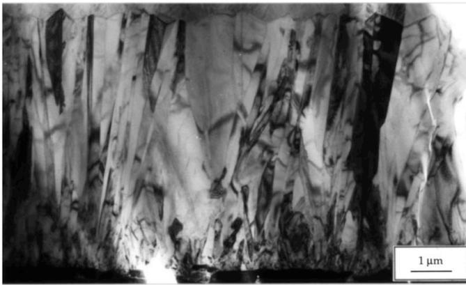
**Figure 4.** TEM image of the microstructure of  $\text{TiC}_x\text{N}_{1-x}$  coating<sup>33</sup>. This image is in cross section view with the substrate at the bottom. This image was reproduced from reference 33.
