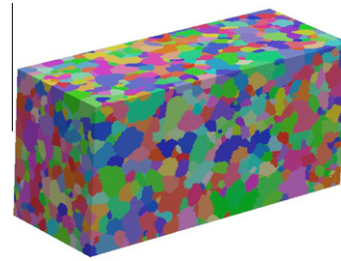
Figure 1. Inverse pole figure of IN100 with twins removed. It comprises 1818 bulk grains and 398 × 146 × 184 voxels, with 1 voxel = 0.25 μm.
