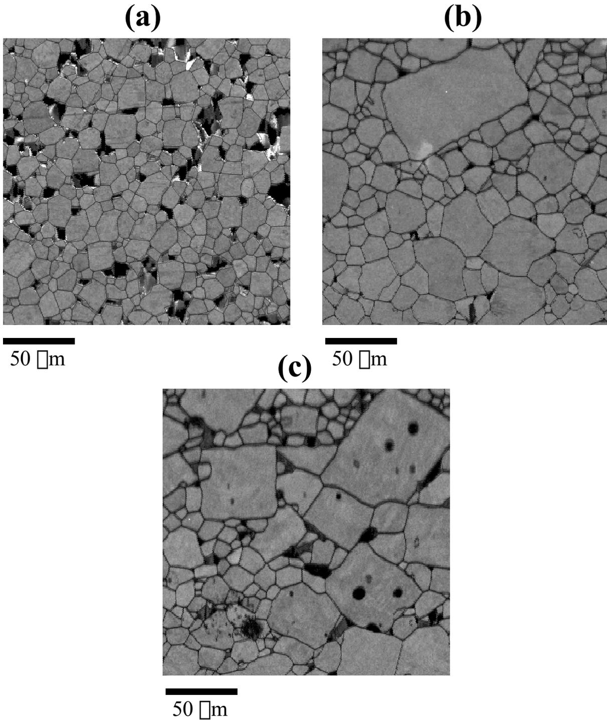
**Figure 1.** OIM image quality maps of matrix grains in PMN-35PT + 1.5 vol% PbO annealed for (a) 0 hrs, (b) 2 hrs, and (c) 4 hrs showing that the morphology is mostly faceted.
