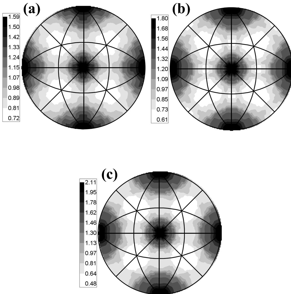
**Figure 3.** Stereograms of PMN-35PT + 1.5 vol% PbO annealed for (a) 0 hrs, (b) 2 hrs, and (c) 4 hrs showing the distribution of interfaces in each sample.
