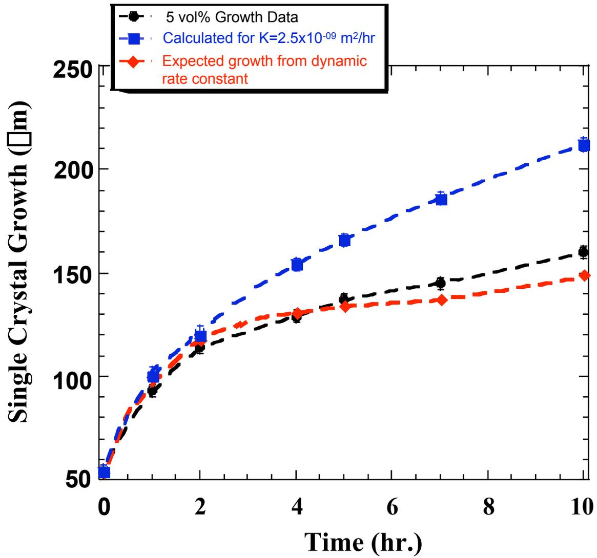
**Figure 2.** Plot of single crystal growth versus time for PMN-35PT + 1.5 vol% PbO including the calculated ideal crystal growth.
