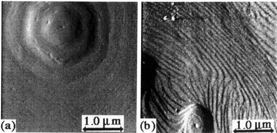
**Figure 2.** Growth hillocks on the surface of a flat facet on the GaN epilayer. These SFM images were recorded based on the difference between the setpoint deflection and the actual deflection of the probe so that contrast corresponds to changes in the topography. This allows a large dynamic range of height data to be viewed simultaneously. (a) shows one of the larger hillocks and (b) shows a smaller one in the lower portion of the image and single layer steps elsewhere.
