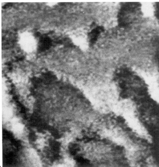
FIG. 1. 1000 \times 1000 \text{ \AA} area of the cleaved CTB (001) surface showing a flat, terraced surface area. The vertical distance from black-to-white is 15 \text{ \AA} .
