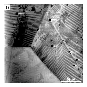
Atomic Force Microscopy (AFM) was used to study the as-polished surface of polycrystalline  $BaTiO_3$ .  $BaTiO_3$  exhibits two different types of ferroelectric domains, named for the relative positions the polarization vector across the domain wall. 90 domain walls lie on a (110)-type plane and are straight while, 180 walls are not restricted to a particular habit plane and typically appear "curvy".
