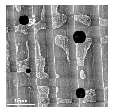
Atomic Force Microscopy (AFM) was used to determine the photochemically active ferroelectric domains in  $BaTiO_3$  by combining established probe reactions with known acid etch techniques. As-received {001} oriented single crystals were heated to 150 C for 10 minutes in air and then cooled to produce a domain structure.
