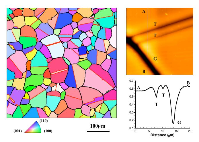
Electron backscattered diffraction mapping was used to create the orientation map (above left) which shows a large concentration of twins in a Nb<sub>2</sub>O<sub>5</sub>-doped TiO<sub>2</sub> sample treated at 1100°C for 24 h in air. The twins appear as straight boundaries, occur on {101} planes, and correspond to boundaries with a 66° rotation about [100]. In the orientation map, twin boundaries are colored red, while general boundaries are black.
