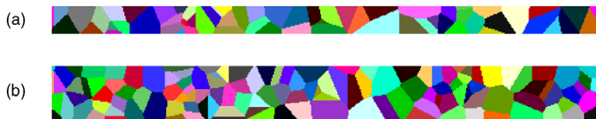
Fig. 3. The microstructures corresponding to nucleation in films having (a) \bar{h} = 1.8 and (b) \bar{h} = 3.5 , respectively. The boundary conditions alter the distribution of grain areas relative to that of an infinite system.
